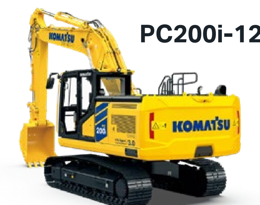
New-generation hydraulic excavator, 3D machine guidance as standard feature
